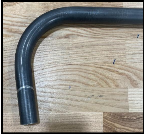
Tube with a short leg and a 'Scribe' line.
