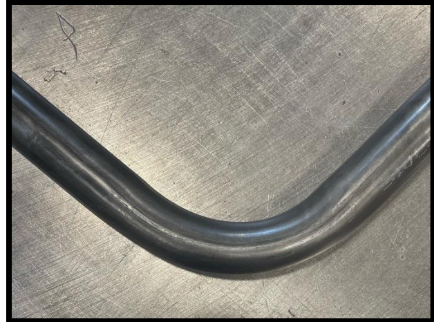
Tube with 'Flattening' due to a tight radius and thin wall.
